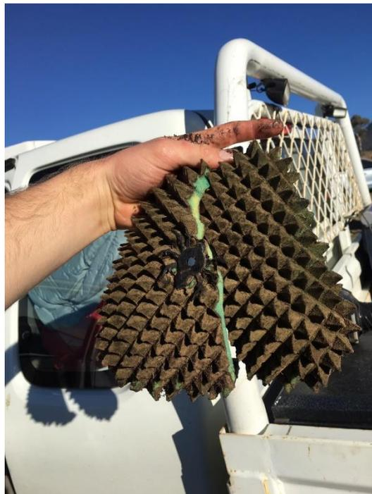
Air filters trap dirt to protect the engine.
